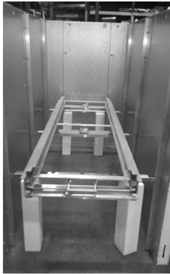
Figure 12: View of raised tray assembly on temporary supports.
